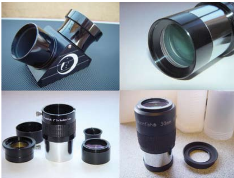
The accessories that arrived with the telescope in the foam lined case were: 2" dielectric diagonal (top left), 2X 2" barlow lens (top right and bottom left) and 30mm 2" Ultrawide eyepiece (bottom right)
