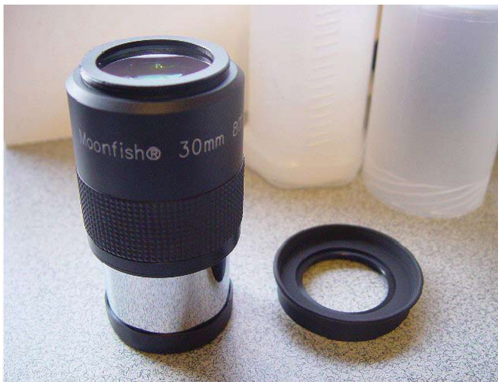
The 30mm 2" Moonfish Ultrawide is listed as being a five element eyepiece, the elements being in three groups and fully multi-coated.
