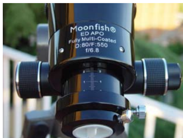
The telescope features a dual speed Crayford type focuser with an 11:1 gear ratio for fast and fine focusing. Note the focus repeatability scale etched onto the drawtube.
