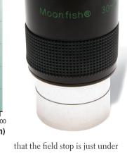
that the field stop is just under 41mm in diameter. Our tests revealed that figure to be 44.8mm, delivering a staggering 4.3° field with the Tele Vue-85 refractor. The view was coma-free out to 70-75 per cent of the field radius with good contrast and colour correction.
